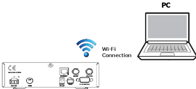
Figure 25 : ACU to PC Wi-Fi Connection
